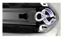
3. Attach the tow chain to the towing eye.
