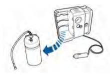
**4.** Insert the new canister and replace the cover.
