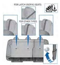
RUN THE TETHER STRAP OVER THE CENTER OF THE HEAD SUPPORT EXCEPT WHEN INSTALLING A LATCH-RETAINED. (ISOFIX-RETAINED) CHILD SAFETY SEAT IN THE CENTER
