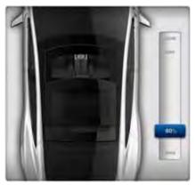
Touch **OPEN** once to open the sunroof to its comfort position (80% open to minimize wind noise). Or, move the sunroof to the comfort position by dragging the slider bar to the indent position. If you find wind noise (which varies depending on driving speed) excessive, even with the sunroof in the comfort position, open a window slightly.
