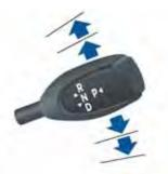
If you try to shift into a gear that the current driving speed prohibits, you hear a chime and the gear does not change.
