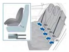
Once installed, test the security of the installation before seating a child. Attempt to twist the child safety seat from side to side and try to pull it away from the seat, then check that the anchors are still securely in place.
