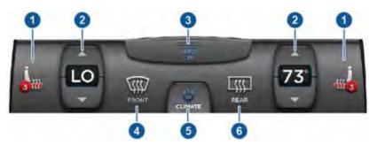
The front seats are equipped with heating pads that operate at three levels from 3 (highest) to 1 (lowest).
