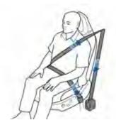
If the pre-tensioners and airbags did not activate in an impact, this does not mean they malfunctioned. It usually means that the strength or type of force needed to activate them was not present.
