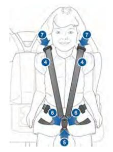
To release, press the button on the buckle, and separate the two halves of the seat restraint.
