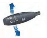
The turn signals stop operating when canceled by the steering wheel, or when you return the lever to the central position.
