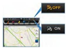
You can also turn the passenger airbag on or off by touching the status indicator, shown above.
