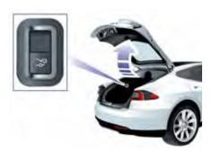
If Model S is equipped with the optional tech package, you do not need to push it up. When you press the release switch, it opens, and when you pull the switch, it closes.
