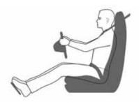
Position the seat so you can wear the seat belt correctly, while being as far away from the front airbag as possible:
